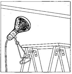
Heat lamp. If the suspected ice blockage is behind a wall or otherwise out of reach, set an electric heat lamp nearby. Keep it at least 6 inches from the wall to avoid scorching paint or wallpaper. For greater flexibility in handling, you can screw the bulb into the socket of a portable work lamp. Pipes that disappear into the ceiling can also be thawed with a heat lamp; hang the lamp directly below the frozen section.
